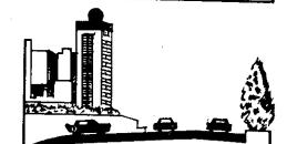
street grades should be flattened out within 100 feet at intersections
